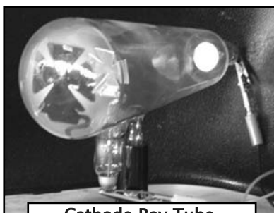
Cathode Ray Tube, ancestor of the TV set.
