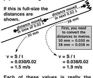
Each of these values is really the <u>average</u> speed over the time and distance between dots. However, this is such a short time period that it is taken to be the <u>instantaneous</u> speed.
