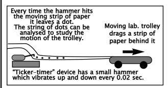
When the trolley moves, it drags the paper through the "ticker-timer" device. A small hammer hits the paper every 0.02 second and leaves a dot. The string of dots is a record of both distance and time over very short time intervals. Here is an example of what part of the paper record might look like.
