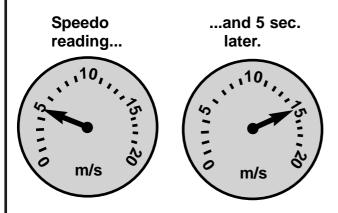
In 5 seconds it has accelerated from an <u>initial speed</u> of 5 m/s to a <u>final speed</u> of 15 m/s. This means that the speed increased by 10 m/s, over 5 seconds.
