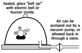
When the bell-jar is filled with air, you can clearly hear the bell ringing.
