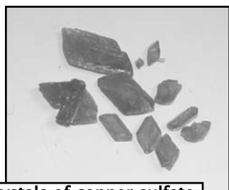
Crystals of copper sulfate collected from a solution by evaporation
